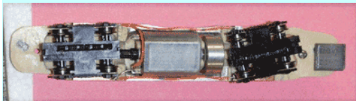
Figure 4 - Running gear installed and wired.
